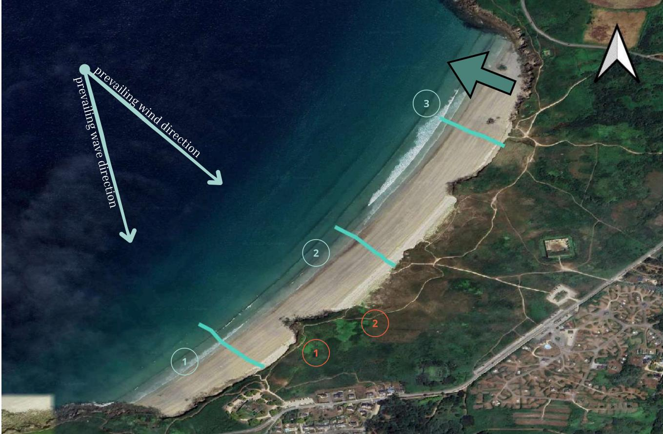
Site surveyed using leveling profiles to capture beach topography.
