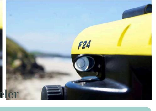
A leveler is a tool to assess beach slope. This is done by moving along a straight line with a giant ruler, while another person is looking through a telescope at a fixed angle of 0 degrees. Relative to the position of the telescope, the height is then measured along the line.
